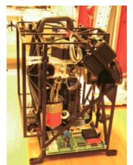
Prototype of an instrument for the detection of biomolecules in interplanetary exploration.
