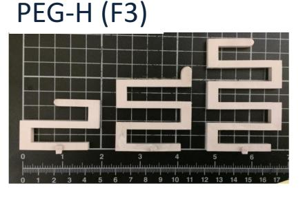
Meander is a complex shape to be injected. Complete samples were injected from all the feedstocks
