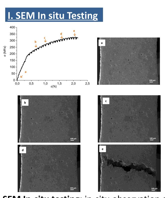
**SEM In-situ testing:** in-situ observation of fracture and further fractography
