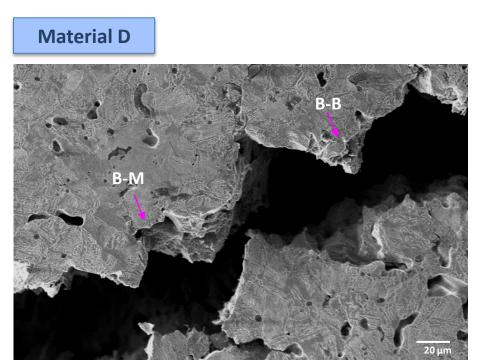
✓ Crack nucleation: Bigger pores (~ 400-700 µm²) and soft phases
