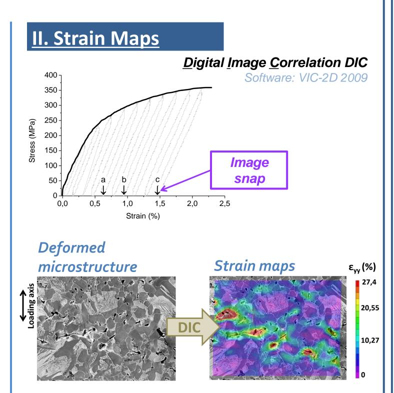
**Strain maps:** evolution of local plastic deformation during tensile testing
