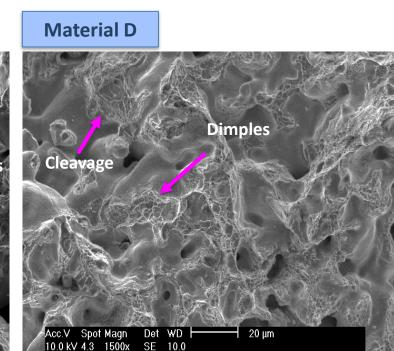
The observed micromechanisms of fracture confirms preferential crack path
