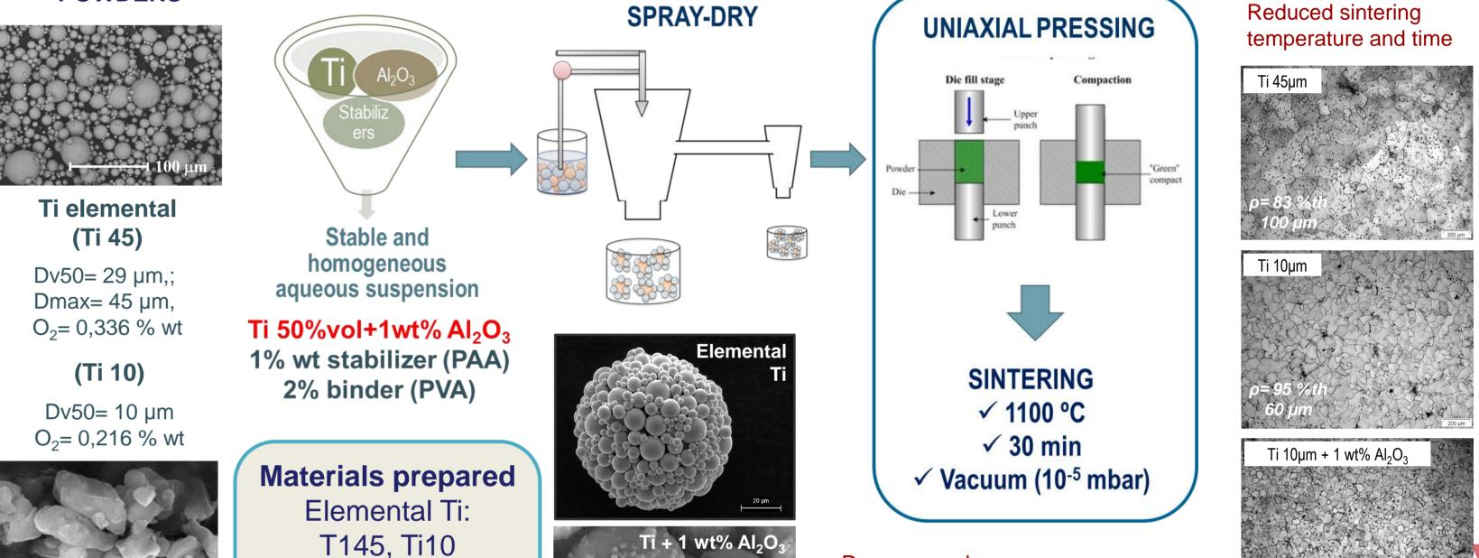
Dense granules High packing of particles Size distribution: 30 – 300 µm Homogeneous dispersion of ceramic particles High compressibility
