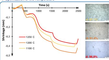
Sintering conditions: 50 C/min – 50 Mpa applied at 600 C – Under vacuum
